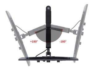
The bracket can be rotated to 90° both left and right.
